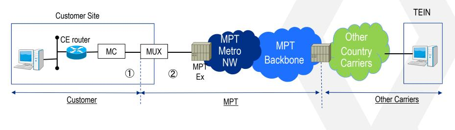
1 In-house cable need to be provided and installed by Customer
